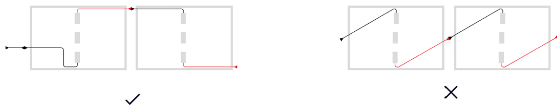
Figure 31 Daisy-Chain position and interconnection for landscape modules.
